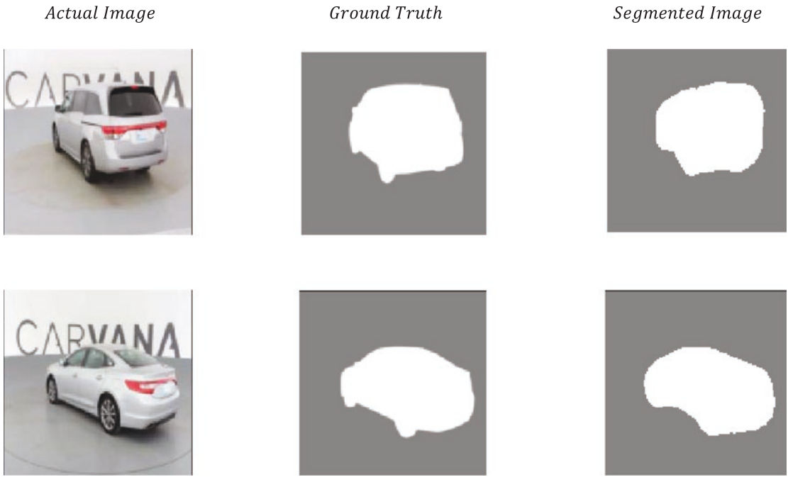
Figure 6-15a. Segmentation results on the validation dataset with model trained on 128×128 -size images
