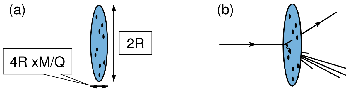
Fig. 2.7: In the Breit frame, the proton of diameter 2R is contracted to a pancake of thickness 4RxM_p/Q (a) so that a photon of high virtuality Q interacts incoherently with a single parton within it (b)
