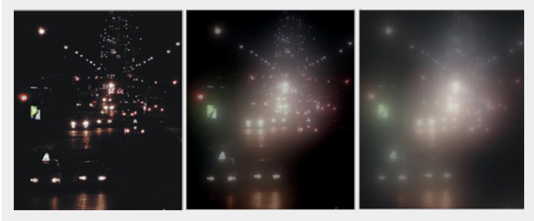
Fig. 29: Multiple scattering (diffusion) of light passing through a wetter and wetter windscreen (left to right).
