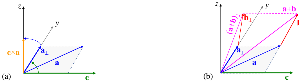
Figure 16.3 (a) Construction of a cross product. (b) The cross product of a sum: The projection of \mathbf{b} slides its tip to the y - z plane.
