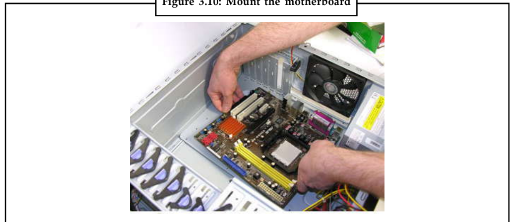
Figure 3.10: Mount the motherboard
