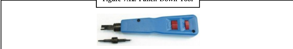
Figure 7.12: Punch Down Tool
