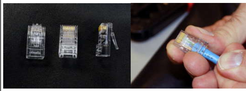
Figure 7.22: Pushing the wires into the connector
