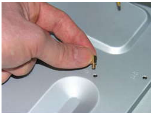
Figure 3.8: Screw Brass Standoffs into The Motherboard
