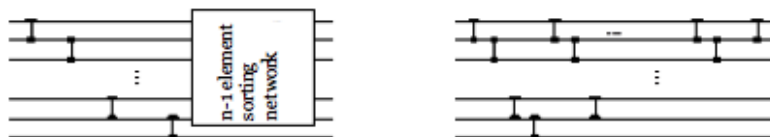
Exhibit 17.18: Selection sort leads by induction to the sorting network on the right.
