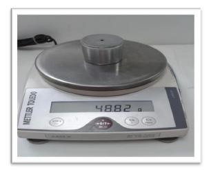
Fig. 8: Pycnometer along with weighing balance
