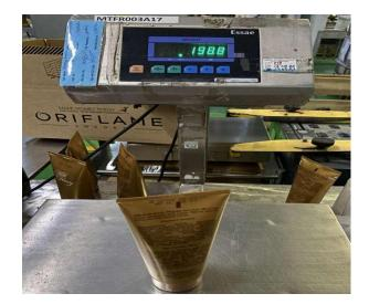
Fig. 18: Checking weight during finish good inspection
