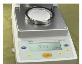
Fig. 11: Weighing of sample to determine Loss on drying
