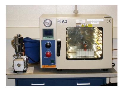
Fig. 19: Vacuum Oven for leakage testing
