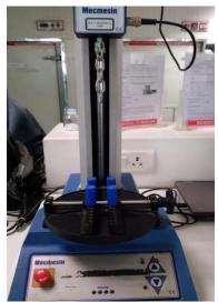
Fig. 21: Universal Testing Machine for foil sealing test
