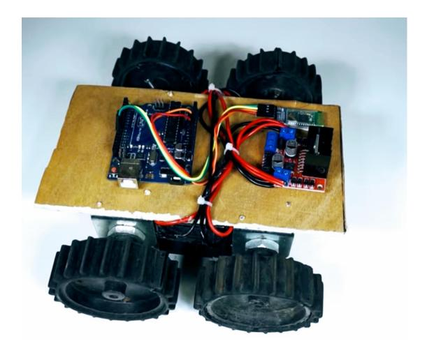
This project presents a simple robotic vehicle which can be controlled using the voice commands over a distance of up to 100m. This allows the user to be able to manipulate the movement of the vehicle wirelessly while maintaining proper distance from the vehicle itself. The vehicle do not require to be trained to adapt to the user's voice and can be operated easily over longer range compared to RF based remote controlled vehicles.
