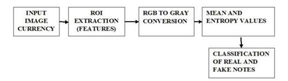
•Figure of Block diagram of the proposed system of image processing.
