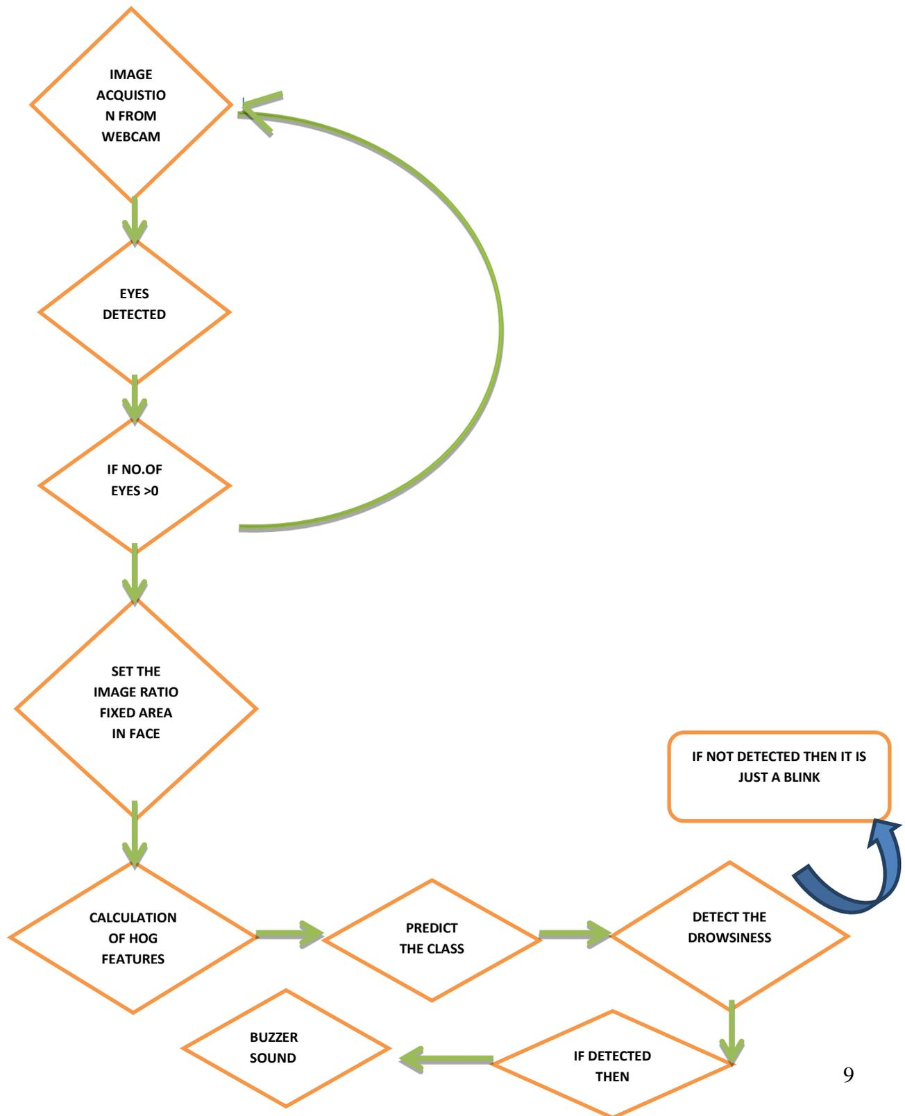
Drowsiness of a person can be measured by the extended period of time for which his/her eyes are in closed state. In our system, primary attention is given to the faster detection and processing of data.
