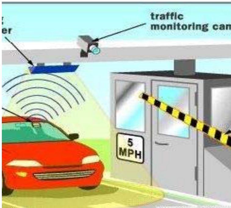
Fig 4. Use of RFID to detect Emergency vehicle
