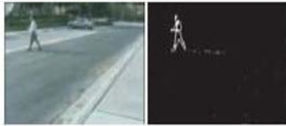
Figure 2-3: Gradient based background subtraction in a certain frame
