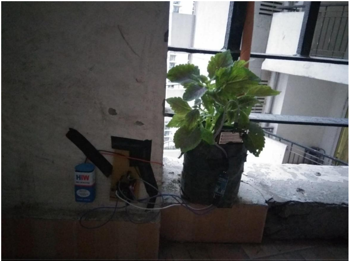
Figure 6: Soil Humidity Sensing
