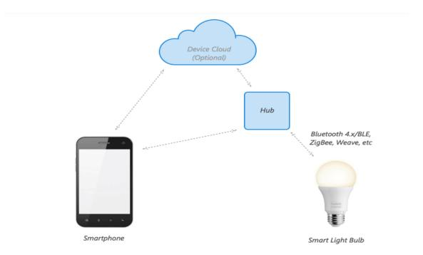
With the hub-centric architecture it is easier to organize the grouping and seamless connection of the many light bulbs and other appliances in a house. Every connected device can be controlled from anywhere and at any time. Background smart triggers, from integrations to the third party services (IFTTT, stock market dynamics, etc), are easily achievable, as well as controlling devices from any smartphone belonging to the home owners.
