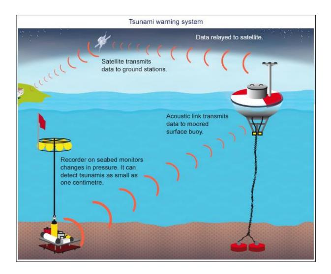
As we can see in the above fig. the data from sensor been transferred to the Buoy and then to the satellite and then to the station or further processing.
