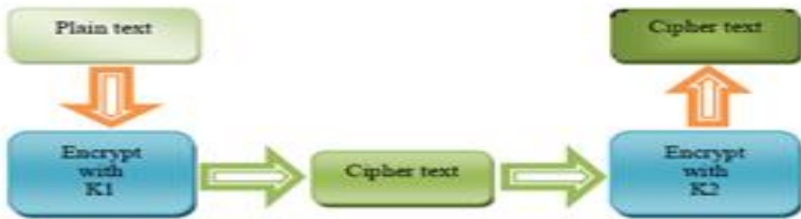
Fig. 2. Encraption process using two keys K1 and K2
