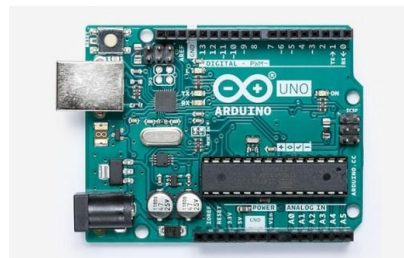
Figure 4. Arduino Uno R3
