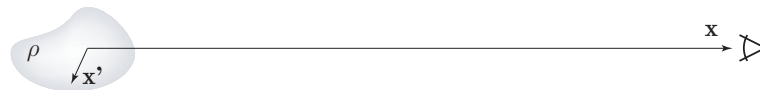
Figure 2.1: A charge/observation point configuration that qualifies for a multipole expansion. Discussion, see text.
