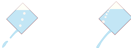
Fig. -13.11. Counter-current flow in a can (the left figure) has only one hole thus pulse flow and a flow with two holes (right picture).
