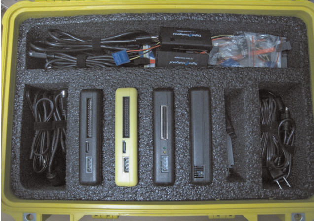
Figure 5.1 Hardware write blockers in a “flyaway” kit.
