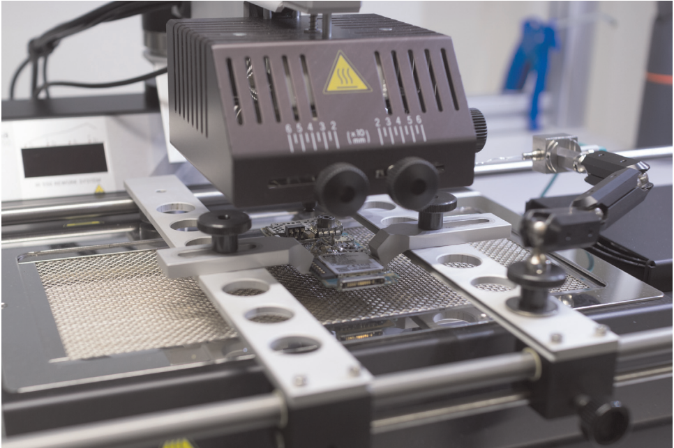
Figure 6.10 An IR rework station with a phone PCB mounted for desoldering.
