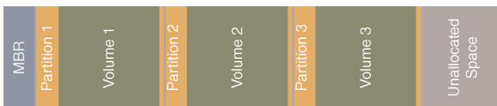
Figure 5.5 Example diagram of partitions on an MBR disk.
