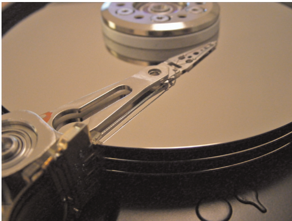
Figure 2.6 A disc from an opened broken hard drive.
