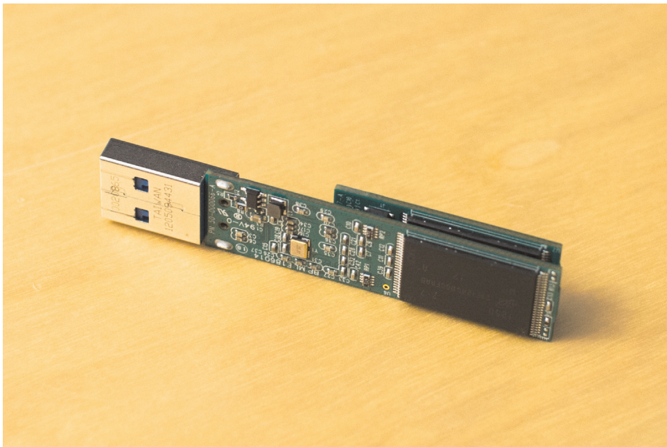
Figure 6.9 A USB memory stick with 4 TSOP packages at the right side of the picture.
