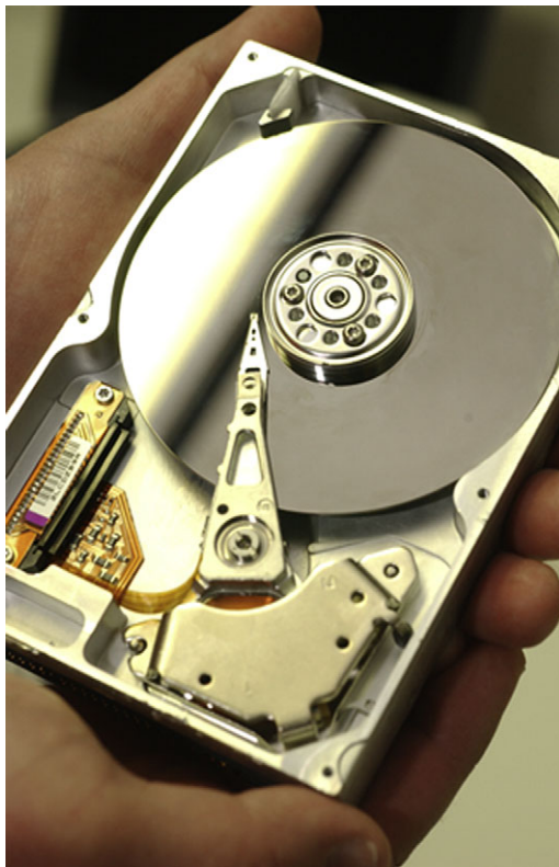
FIGURE 2.3 The inside of a typical magnetic drive.
