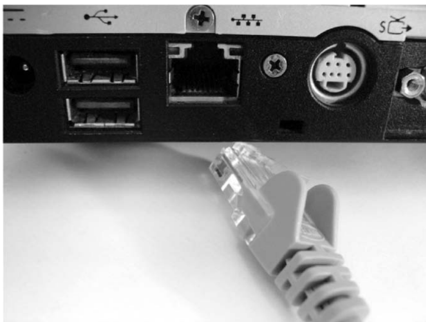
Figure 3.10 A network socket on a PC and associated cable
