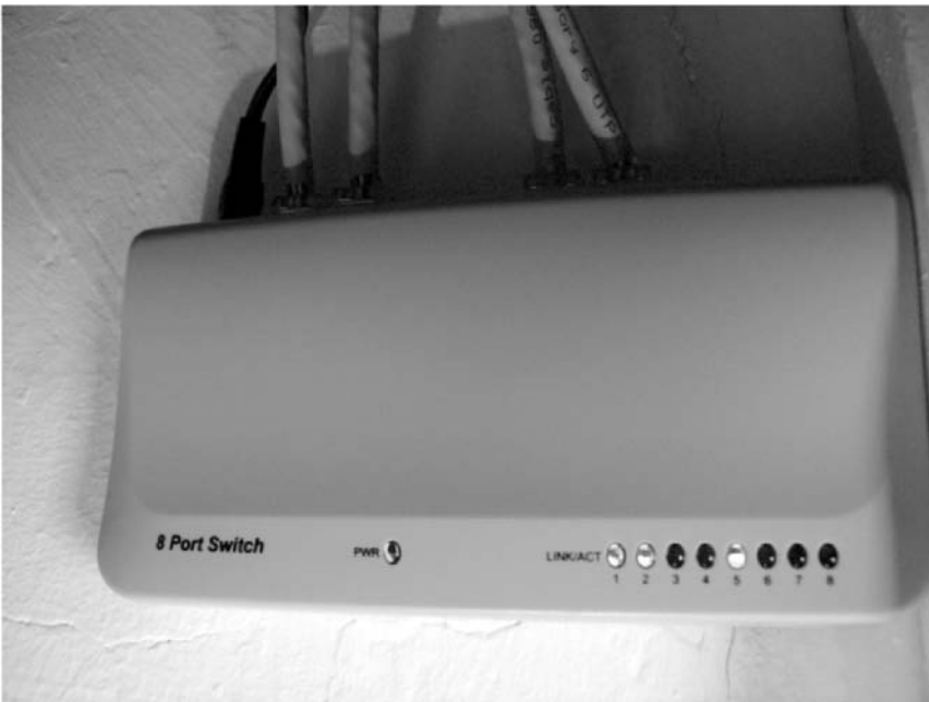
Figure 3.12 A low-cost network switch used to connect multiple machines
