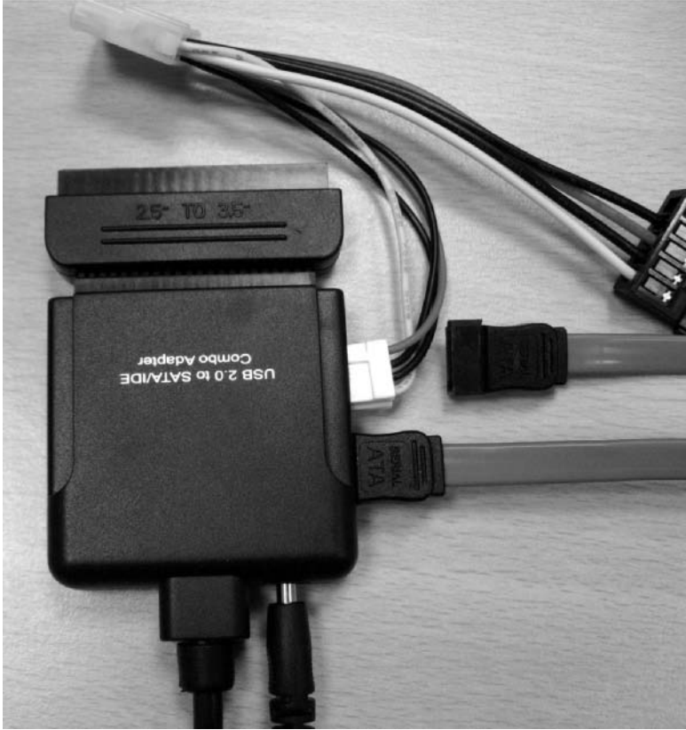
Figure 4.2 A typical SATA/IDE-to-USB hard disc adapter
