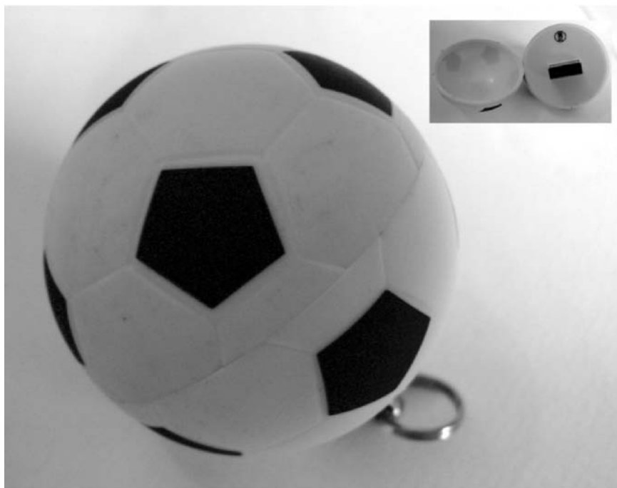
Figure 3.8 A novelty/disguised USB storage device (inset shows the USB connector visible when it is opened)
