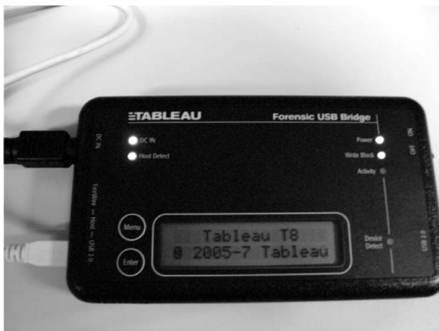
Figure 4.1 A Tableau T8 USB write-blocker used to protect devices against accidental data writing
