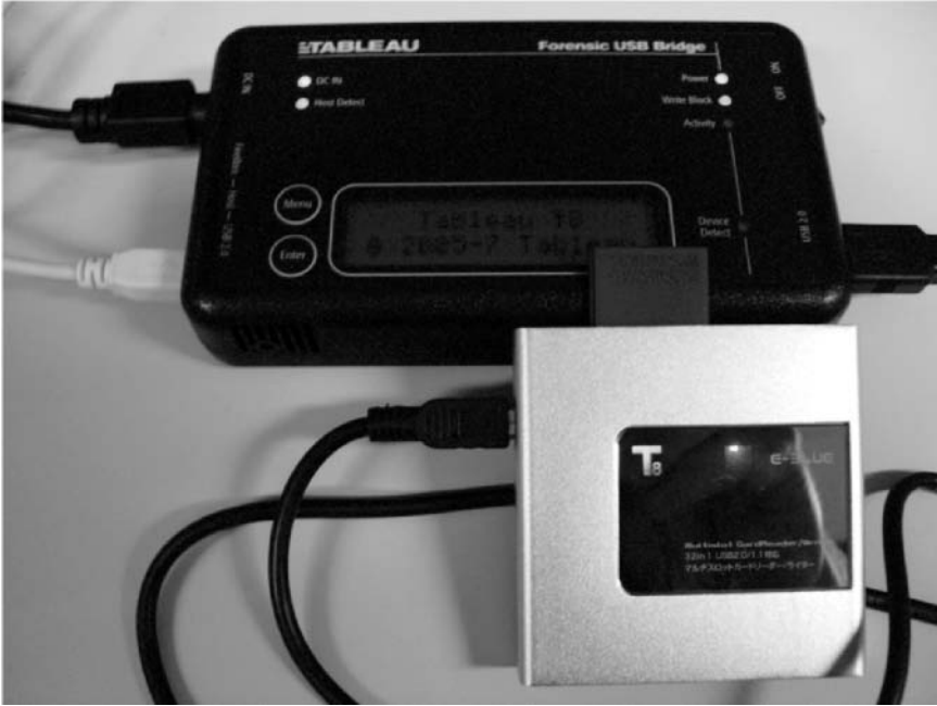
Figure 8.2 A multi-format removable memory card reader connected via a forensic bridge write-blocker
