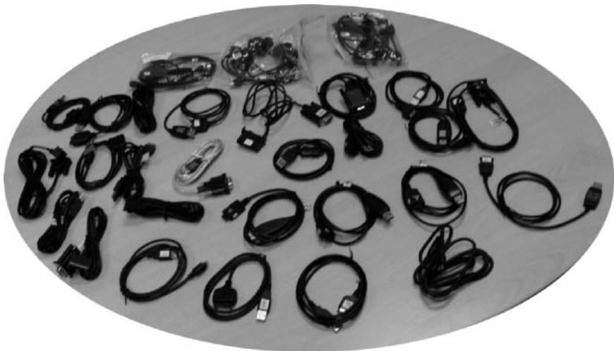
Figure 8.1 A typical set of interface cables found in a mobile device examination kit
