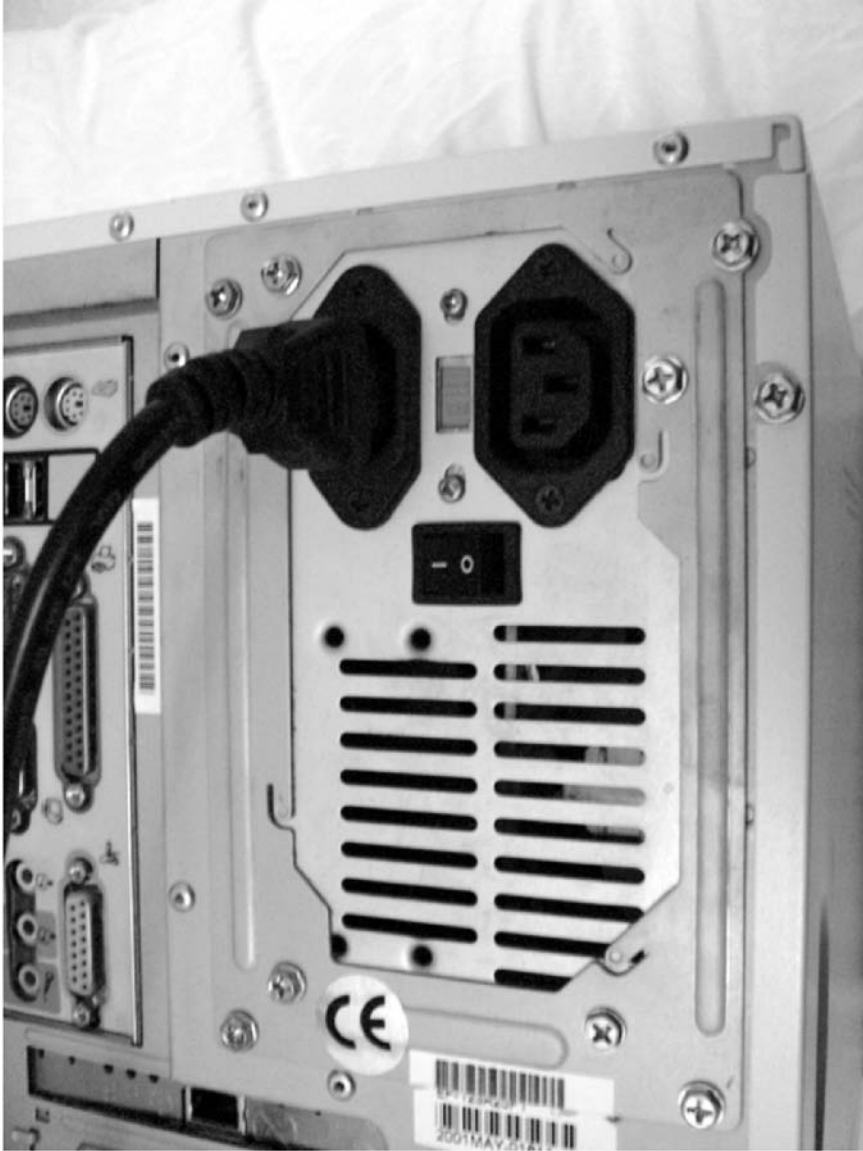
Figure 3.2 A standard power connector on the rear of a PC
