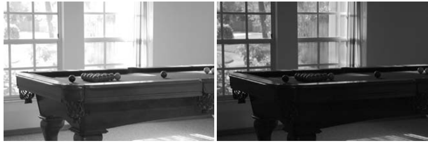
Figure 23.1. With conventional photography, some parts of the scene may be under- or over-exposed. To visualize the snooker table, the view through the window is burned out in the left image. On the other hand, the snooker table will be too dark if the outdoor part of this scene is properly exposed. Compare with Figure 23.2, which shows a high dynamic range image prepared for display using a tone reproduction algorithm.
