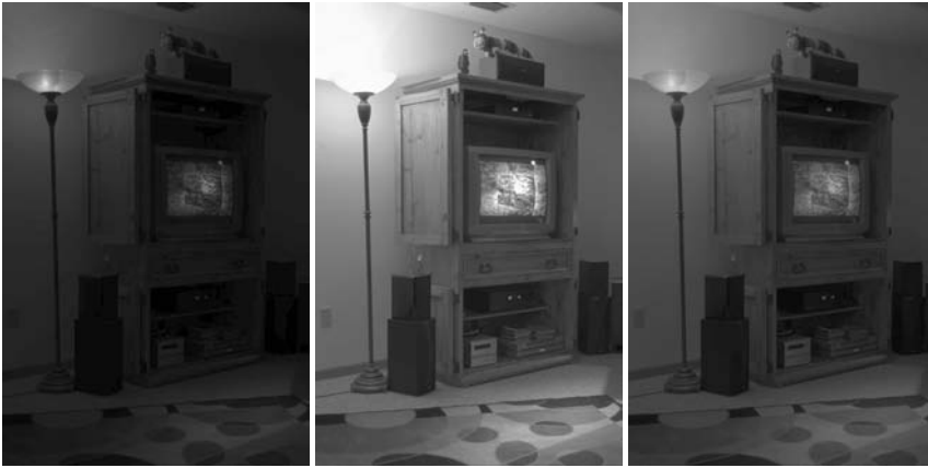
Figure 23.3. Linear scaling of high dynamic range images to fit a given display device may cause significant detail to be lost (left and middle). The left image is linearly scaled. In the middle image high values are clamped. For comparison, the right image is tonemapped, allowing details in both bright and dark regions to be visible.
