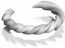
Figure 16.23. Three blended implicit cylinders, twisted together, tapered and bent. Image courtesy Erwin DeGroot.
