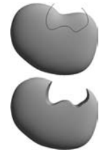
Figure 16.30. BlobTree operations can be applied, e.g., CSG difference. Image courtesy Erwin DeGroot.
