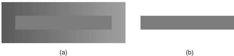
Figure 22.4. (a) Simultaneous contrast: the apparent brightness of the center bar is affected by the brightness of the surrounding area; (b) The same bar without a variable surround.
