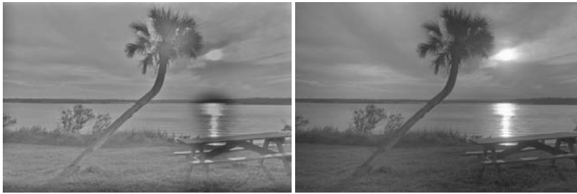
Figure 23.20. Images tonemapped by dividing by Gaussian blurred versions. The size of the filter kernel is 64 pixels for the left image and 512 pixels for the right image. For division-based algorithms, halo artifacts are minimized by choosing large filter kernels.
