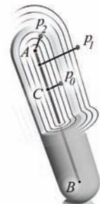
Figure 16.6. Line primitive ab and example points P_0, P_1, P_2 showing distance calculation.
