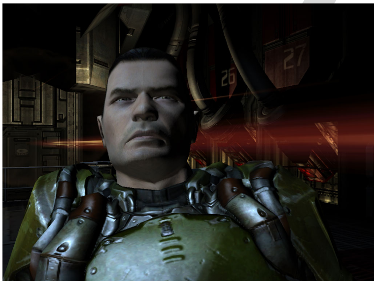
Figure 94 Doom 3 uses unified lighting and shadowing. Shadows are calculated using a stencil shadow volume.
