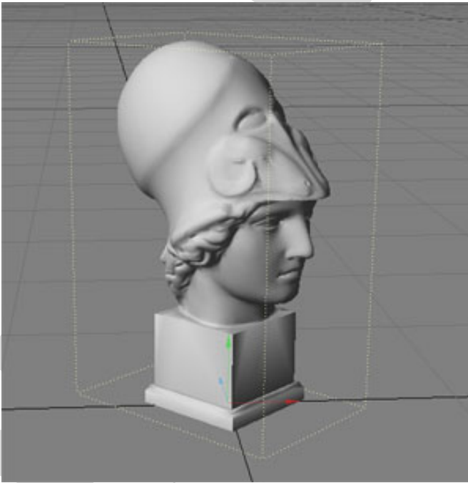
Figure 21 A bounding box for a three dimensional model
