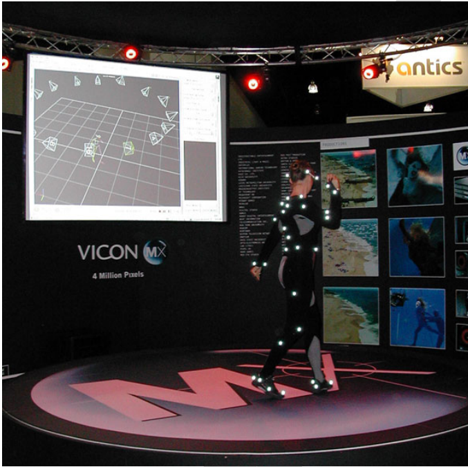
Figure 60 A dancer wearing a suit used in an optical motion capture system
