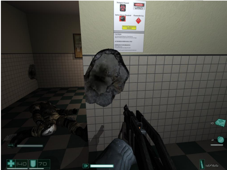
Figure 66 From F.E.A.R., a bullet hole with Parallax mapping used to create the illusion of depth.
