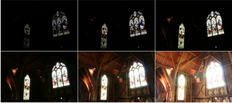
Figure 38 The six individual exposures used to create the previous HDRI. Exposure times from top left are: 1/40sec, 1/10sec, 1/2sec, 1sec, 6sec, 25sec
