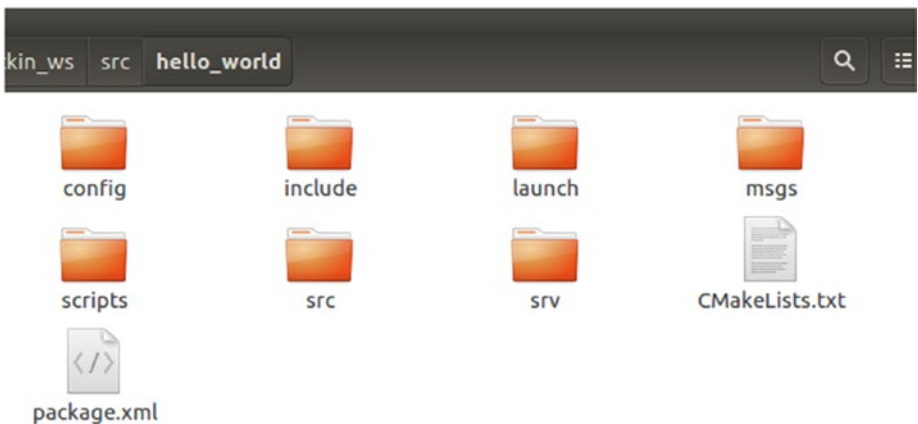
Figure 4-13. A typical ROS package structure
