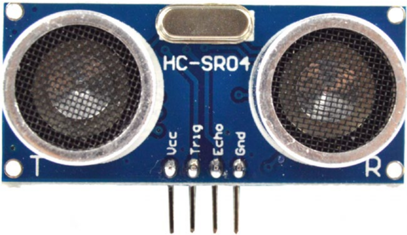
Figure 6-12. The HC-SR04 ultrasonic sensor
