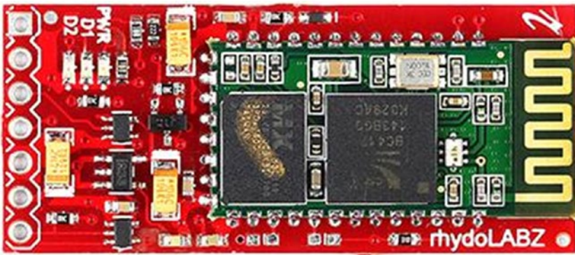
Figure 6-11. The Bluelink Bluetooth module
