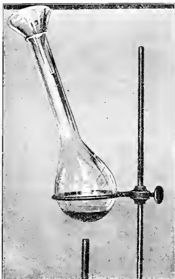
FIG. 24. Kjeldahl flask arranged for the determination of nitrogen
