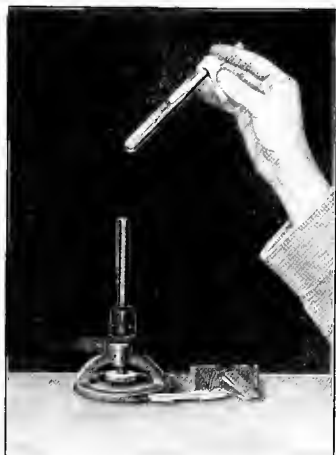
FIG. 21. Showing method of holding splint for the Strobel test
