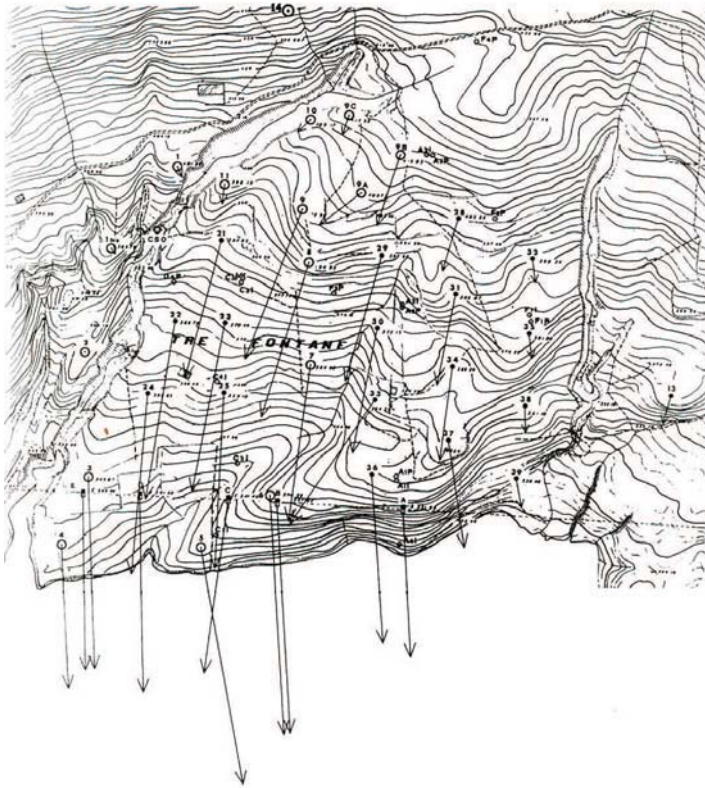
Fig. 99. Planimetry of the landslide in the right bank of the RAGOLETO reservoir and vectors of the average displacements between 1972 - 1994 [100]
