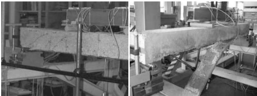
Fig. 2. Breaking mode of reinforced (a) and restored + reinforced beams (b)
