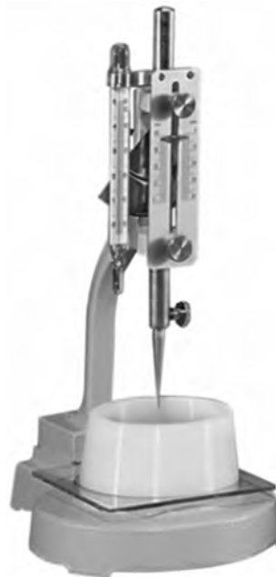
FIGURE 2.1 Vicat needle apparatus to measure consistency of cement.
