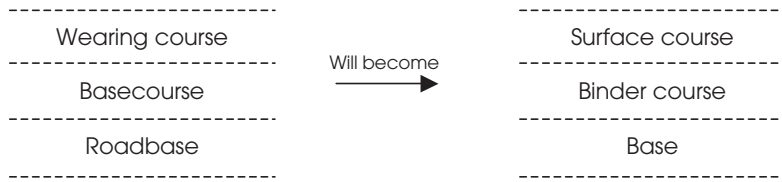
Figure 8.1 Proposed renaming of pavement layers.
