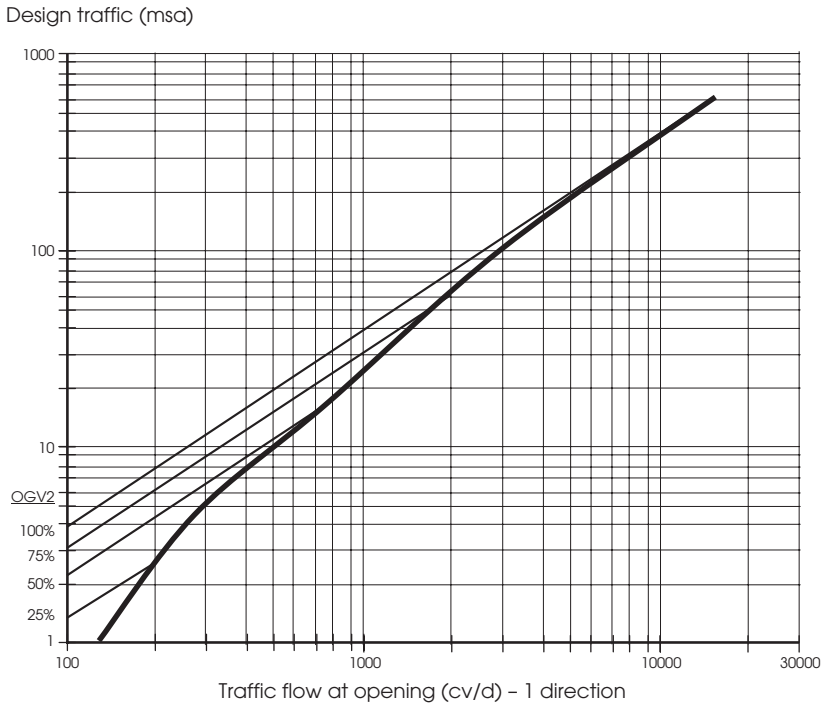
Figure 7.7 Design traffic for flexible and flexible composite pavements (20-year design life) – single carriageway (HD 24/96) (DoT, 1996).
