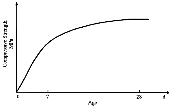
Figure 5.11 The Growth Curve of Concrete's Strength
