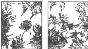
Figure 4.4 The Needle-like Crystals in Cement Paste
