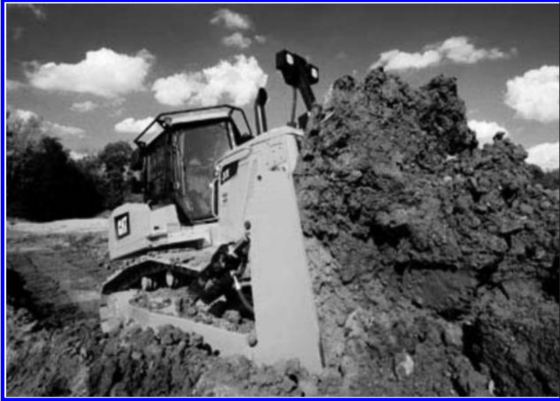
FIGURE 12.1 Caterpillar D7E hybrid-electric dozer. (From U.S. Federal Highway Administration, Part G—Construction Equipment , Washington, DC, Accessed on December 19, 2014, https://fhwaapps.fhwa.dot.gov/nhswt/reader?agency=Delaware&fn=Part+G_Construction+Equipment.pdf&type=manual , 2012.)
