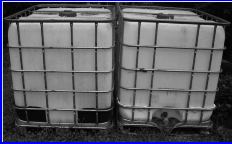
FIGURE E.3 Repurposed intermediate bulk containers for non-potable water storage. (Courtesy of Parker McGee.)
