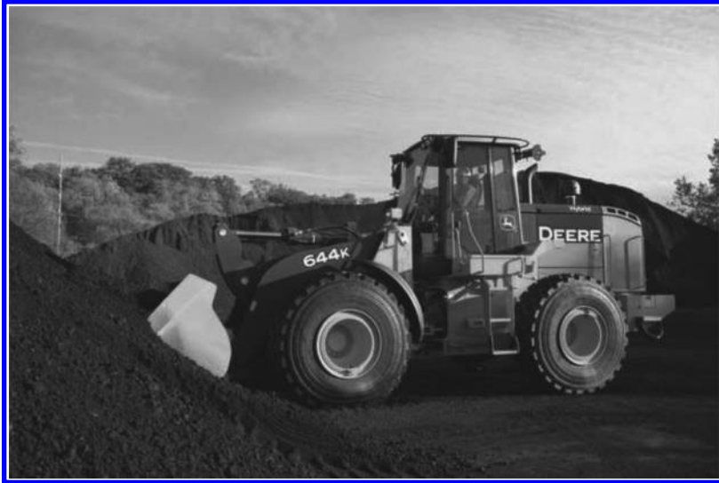
FIGURE 12.3 John Deere 644K diesel-electric hybrid wheel loader. (From U.S. Federal Highway Administration, Part G—Construction Equipment , Washington, DC, Accessed on December 19, 2014, https://fhwaapps.fhwa.dot.gov/nhswt/reader?agency=Delaware&fn=Part+G_Construction+Equipment.pdf&type=manual , 2012.)
