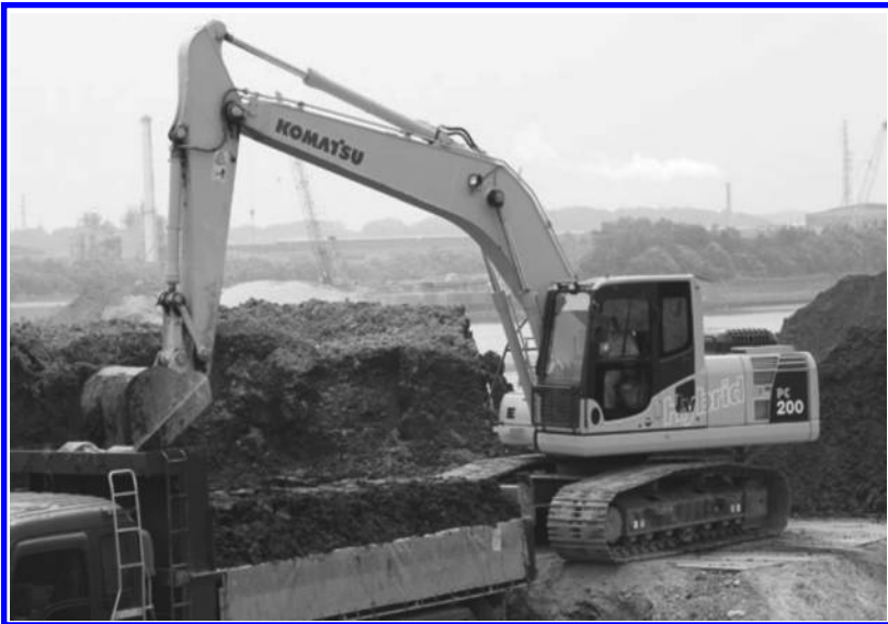
FIGURE 12.2 Komatsu PC200LC-8 hybrid excavator. (From U.S. Federal Highway Administration, Part G—Construction Equipment , Washington, DC, Accessed on December 19, 2014, https://fhwaapps.fhwa.dot.gov/nhswt/reader?agency=Delaware&fn=Part+G_Construction+Equipment.pdf&type=manual , 2012.)
