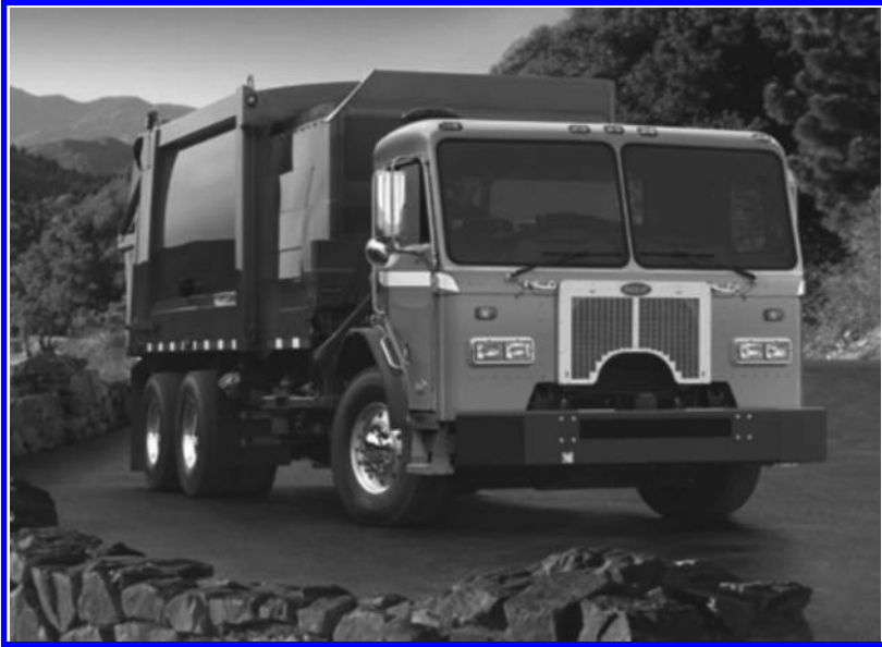
FIGURE 12.4 Peterbuilt model 320 Hybrid Class 8 refuse truck. (From U.S. Federal Highway Administration, Part G—Construction Equipment , Washington, DC, Accessed on December 19, 2014, https://fhwaapps.fhwa.dot.gov/nhswt/reader?agency=Delaware&fn=Part+G_Construction+Equipment.pdf&type=manual , 2012.)
