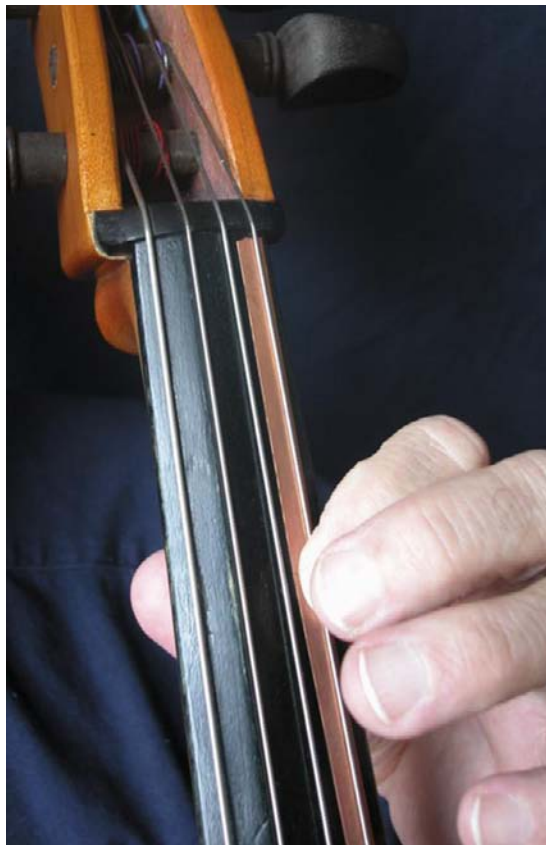
Figure 1. A cellist holds a note using his index finger. The finger placement depresses the string which makes contact with the copper strip affixed to the fingerboard. The string circuit measures the resistance of the string between this point of contact and the bridge.
