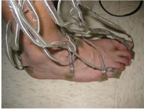
Figure 12. Lateral view of pressure sensors attachment (top right).
