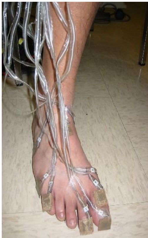
Figure 11. Anterior view of pressure sensors attachment (left).
