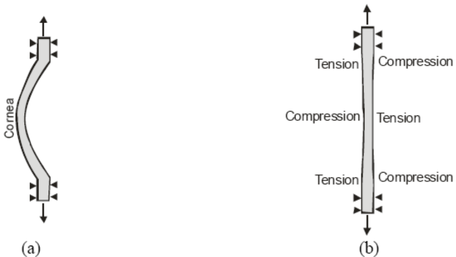
Figure 12. Straightening of (a) an initially curved strip specimen produces stresses and strains with the distribution shown in (b).
