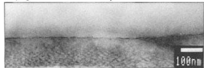
Fig. 2 Cross sectional TEM picture of HS surface 372 days after carotid replacement (from [4] copyright, reprinted by permission of Springer-Verlag)
