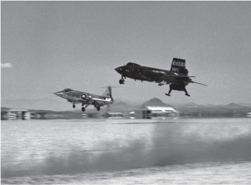
The X-15 lands on the dry lakebed at Edwards Air Force Base, with an F-104 chase plane close by. Smoke canisters provided wind direction data to the pilot. (USAF)
