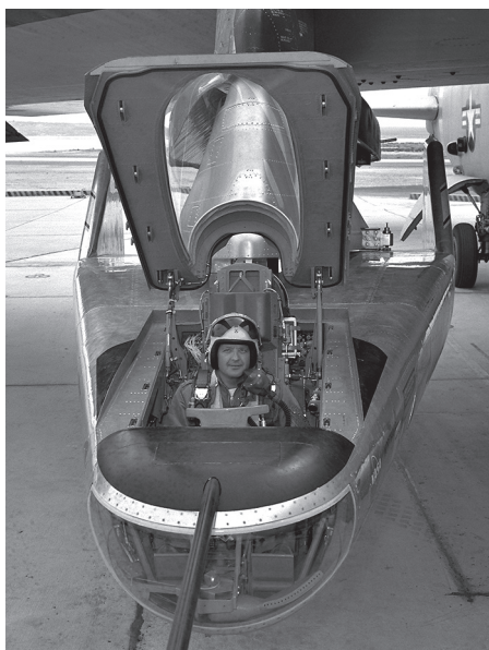
The M2-F2 was carried to launch altitude beneath the wing of a modified B-52. Pilot Milt Thompson endured the confines of the cramped cockpit with a smile. (NASA)
