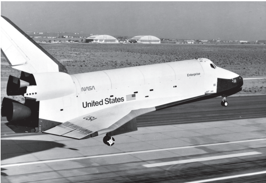
Enterprise approaches the concrete runway at a speed of 200 knots. Pilot-induced oscillation developed during touchdown. (NASA)
