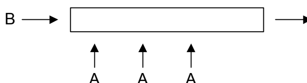
Figure 4a Keeping the reagent concentration low in tubular reactors by small downstream additions of reagent
