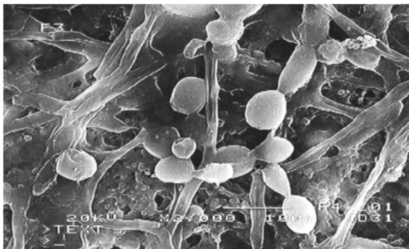
Figure 3. SEM micrograph of the micro-organisms (nonfermenting gram-negative rods) in the deposit collected from the distillate tank walls. Reproduced with permission from [69], Copyright Elsevier, 2005.
