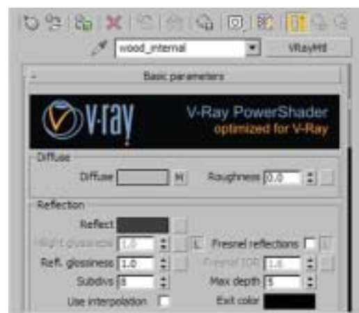
FIG 5.20 Wood Internal, Reflection.
