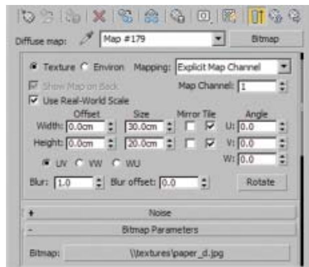
FIG 4.43 Paper Screen, Diffuse Channel, Bitmap Coordinates.
