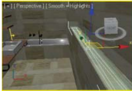
FIG 3.56 Light Recess, Positioning.
