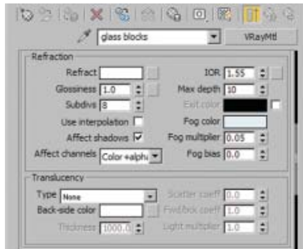
FIG 4.70 Glass Glassblocks, Refraction.
