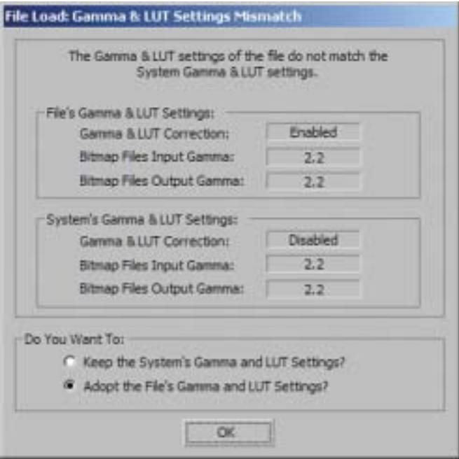
FIG 1.60 File Load: Gamma & LUT Settings Mismatch Dialog Box, Adopt File's Gamma Correction.
