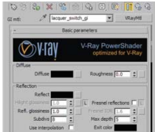
FIG 3.44 Lacquer Switch, V-RayOverrideMtl, GI Material Parameters.
