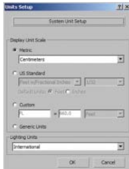
FIG 1.58 Units Setup Dialog Box, Change Units.
