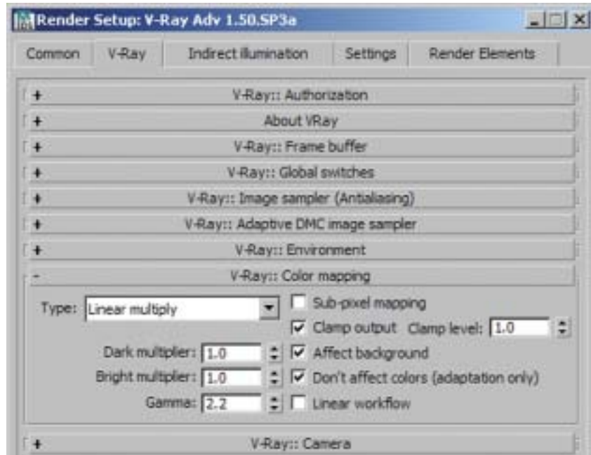
FIG 1.48 Render Setup, V-Ray: Color Mapping, Gamma 2.2, Don't Affect Colors (Adaptation Only).
