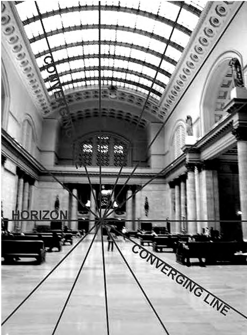
Figure 5.25B A photograph of an interior space depicting a normal-view one-point perspective and showing the converging lines and horizon (source: Randy Sarafan).
