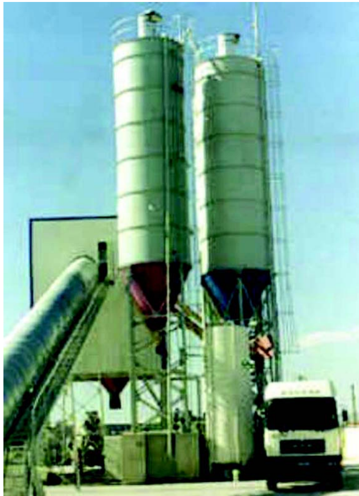
Fig. 10.2 Vertical Batching Mixing Plant
