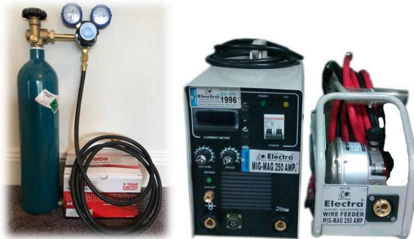
Figure 18: MIG Welding machine & Co 2 cylinder used for AR-20.
