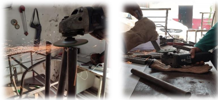
Figure 16: Cutting & Grinding of Chassis Tube,
