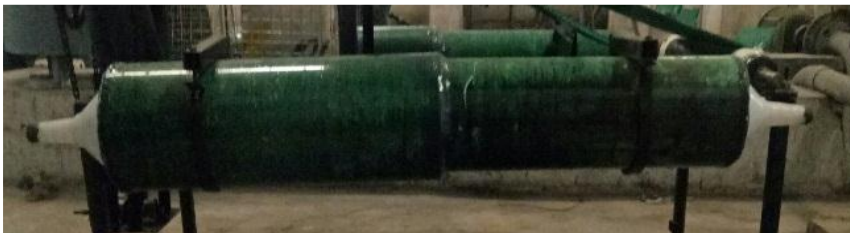
Fig-3.2: Hollow Pipe for floatation
