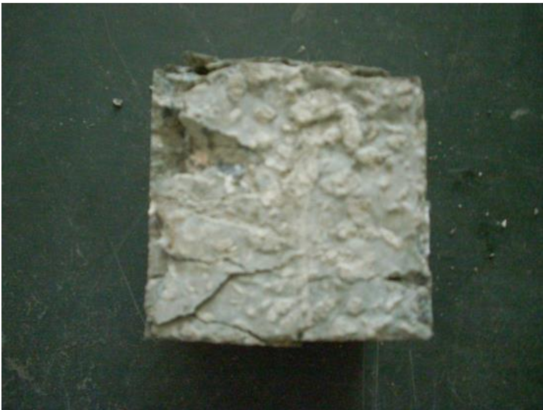
Fig. 3.5(a) Specimen: After Failure at Room temperature.
