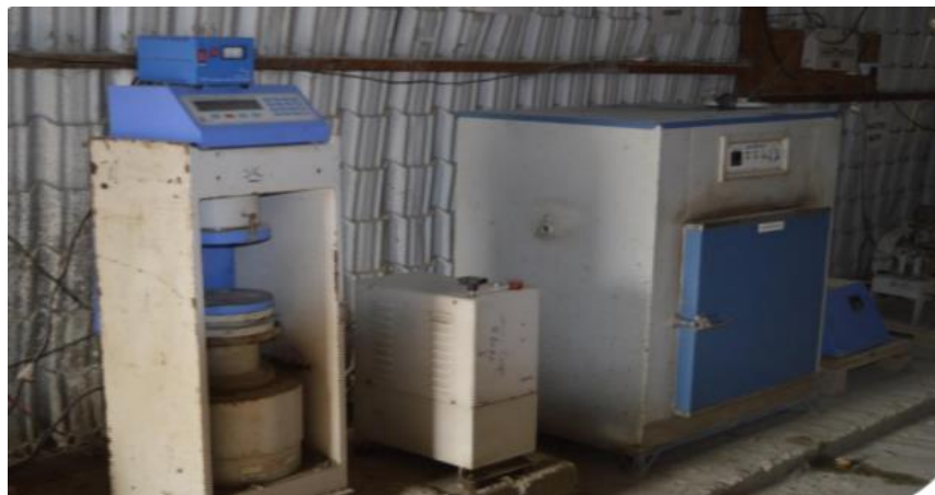
Figure 3.9: (a) Cube Testing on CTM
