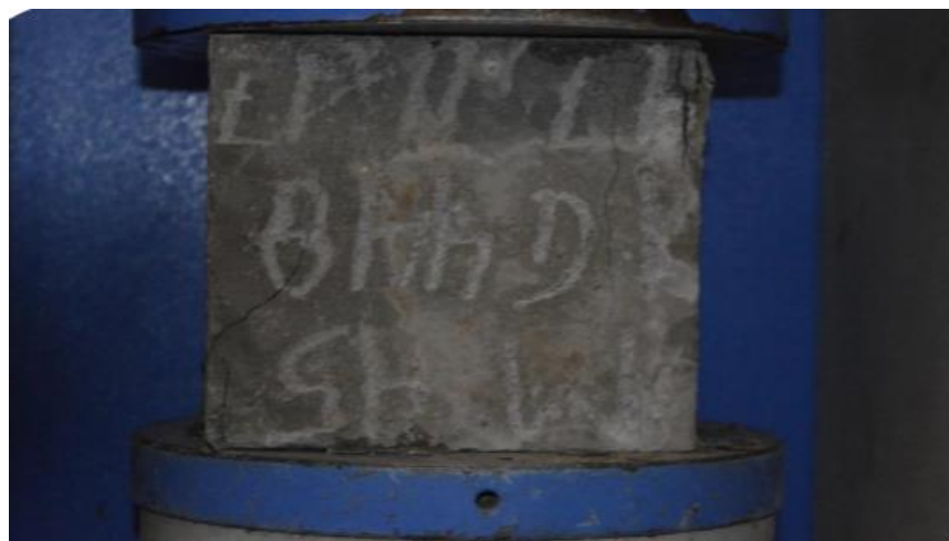
Figure 3.9: (b) Cube Testing on CTM
