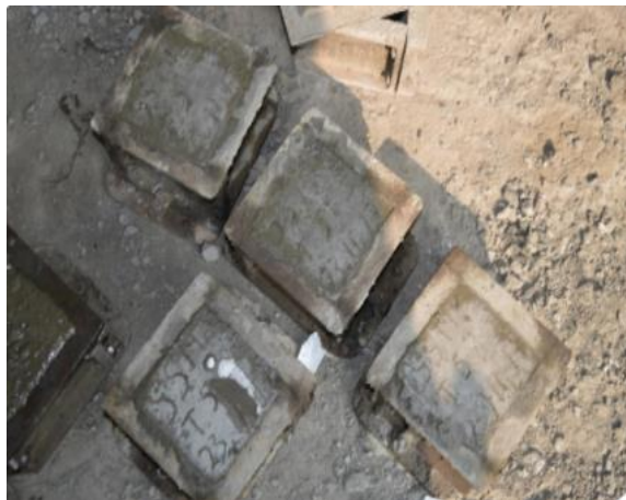
Figure 3.8: (a) Curing of Concrete Cubes
