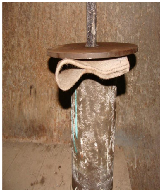
Figure 4. 10 Steel Plate and Geo Textile Membrane Used for Uniform Loading
