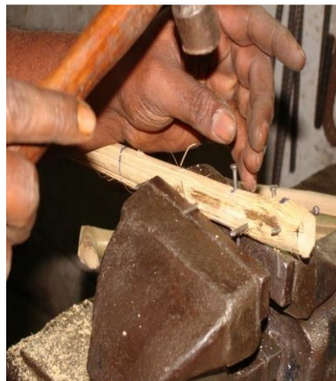
Figure 4. 8 Hammering the Nails through the Holes,
