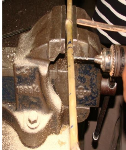
Figure 4. 7 Making Hole by Using Drill Machine,
