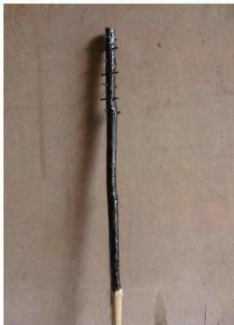
Figure 4. 9 Finished Bamboo Sample (Coated with Tar and Pierced Nail)
