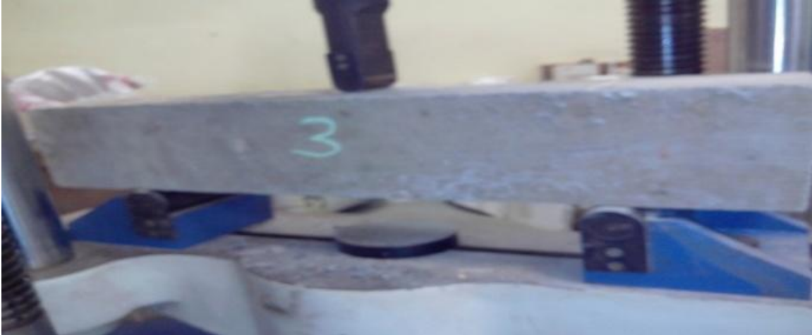
Figure 4.3 Actual Beam under 3 point bending.
