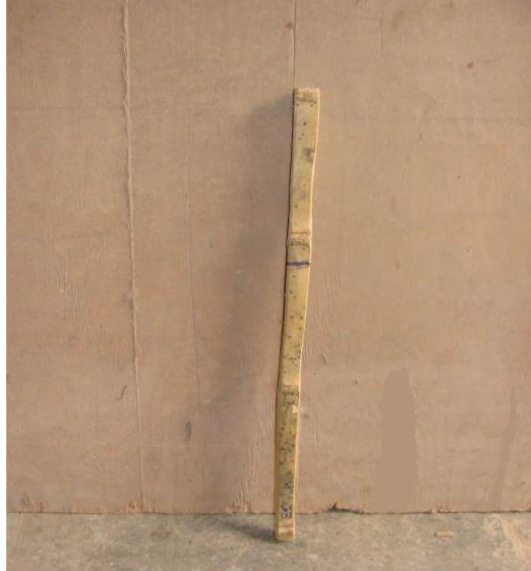
Figure 4. 5 Bamboo Sample (In Natural Condition) for Pullout Test.
