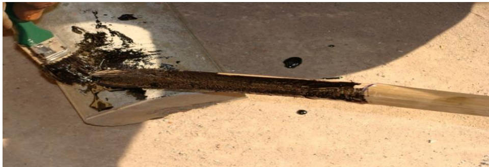
Figure 4. 6 Bamboo Sample Coated with Tar
