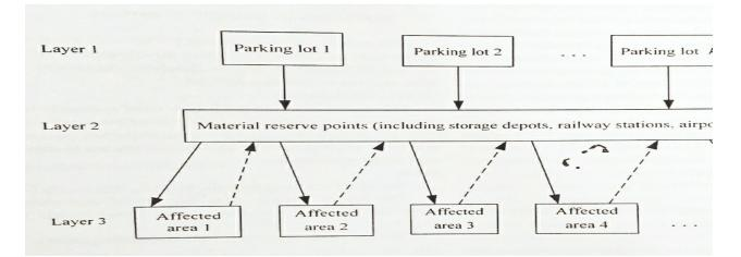
Layer I contains the parking lots; vehicles which are allocated to transport help materials start from this area.
