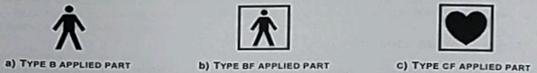
Figure 1 – Symbols indicating the degree of protection provided by an APPLIED PART
