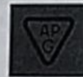
b) Category APG Equipment designed to avoid ignition of FLAMMABLE ANAESTHETIC MIXTURE WITH OXYGEN OR NITROUS OXIDE
