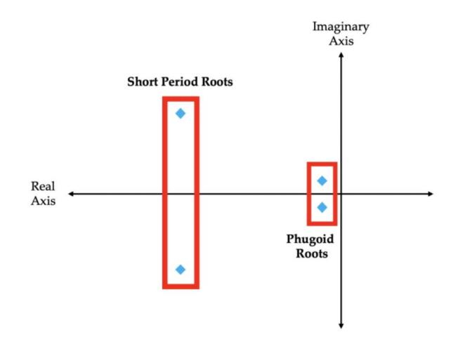
Figure 2: Pole locations describing the longitudinal dynamics of an aircraft
