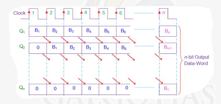
Output Waveform of *n*-bit Right-Shift SIPO Shift Register
