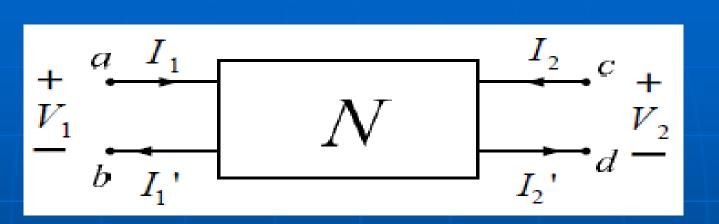
No external connections exist between the input and output ports.
