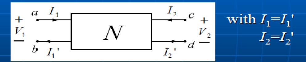
Then terminals a , b constitute the input port and terminals c , d constitute the output port.
