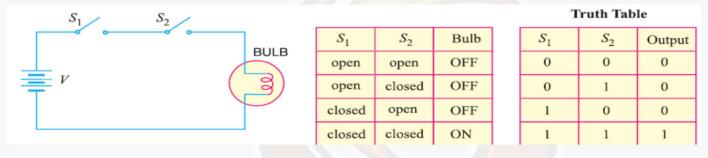
(i) When S1 and S2 are open, the bulb is OFF.
