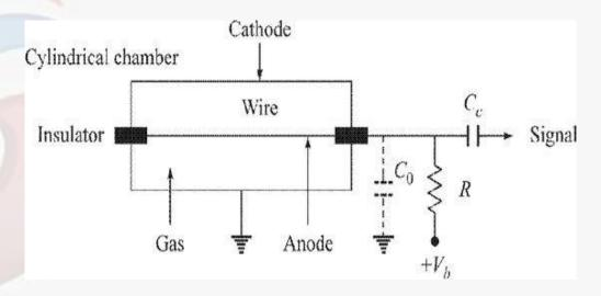
In ionization an electron-ion pair is created. The electrons so liberated when they reach the anode give information that a radiation has entered the detector.
