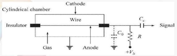
•If there is no electric field present, i.e.  $V_b = 0$ , the ion-pairs just created recombine forming neutral atoms/molecules.
